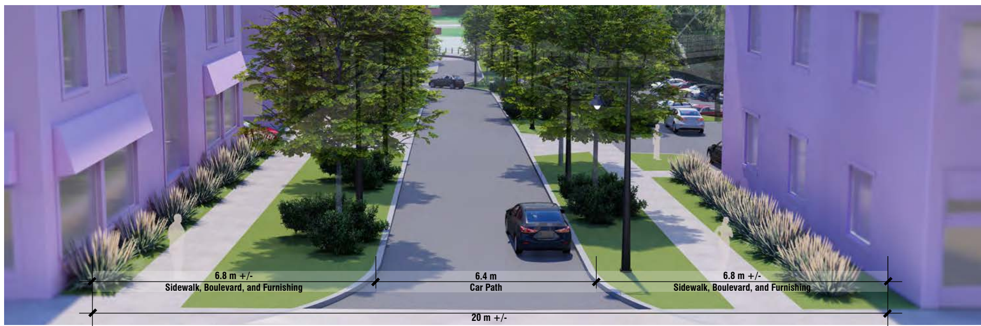
Fig.27: 20m ROW Cross Section Without Street Parking - Market St.
